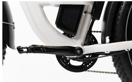
Left pedal (2) tightens anticlockwise
