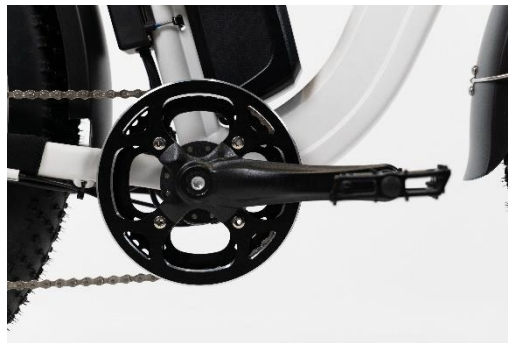
Right pedal (1) tightens clockwise
